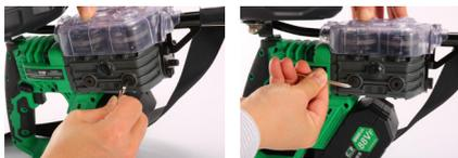
3. Insert the tip of the lubrication tube (provided in the replacement parts kit) and squeeze twice in each hole.
